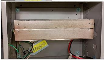
Carefully remove the mounting plate with the power supply attached. Then remove the AC and DC wires from their terminal strip positions. Flip the plate over and change out the defective power supply with the four screws.
