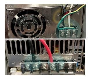
Remount the plate with the new power supply in place using the four 11/32 lock nuts. Reconnect the ground wire to the sidewall. Restore the wire nut connections for AC and DC—power up and test.
