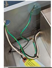
Using the 11/32 socket wrench, remove the four nuts from the mounting plate in the ELT600-24U box so the power supply assembly is free.
